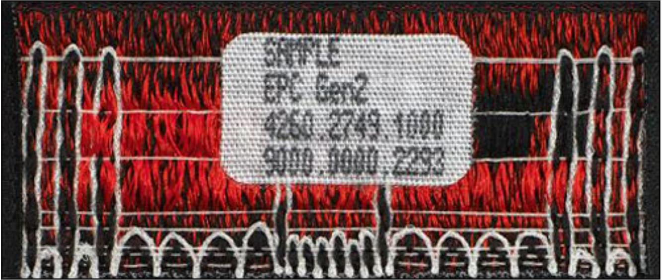
*The backside of TexTrace's RFID label, showing the stitched-in loops of white yarn that serve as the tag's antenna, as well as the rectangular pad that protects the chip.*
